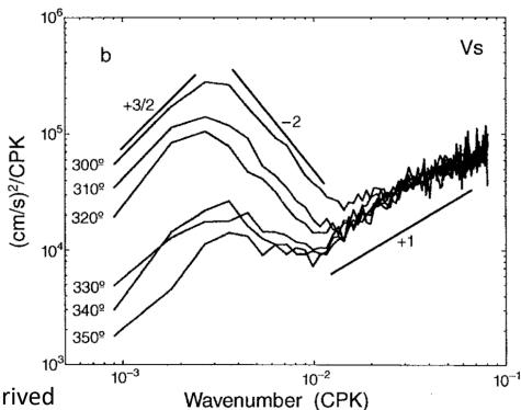
Wavenumber KE spectra of altimeter-derived cross-track geostrophic currents (30N to 40 N)
