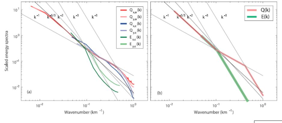
Transition and dissipation scales appear near 10 km and 2 km, respectively
